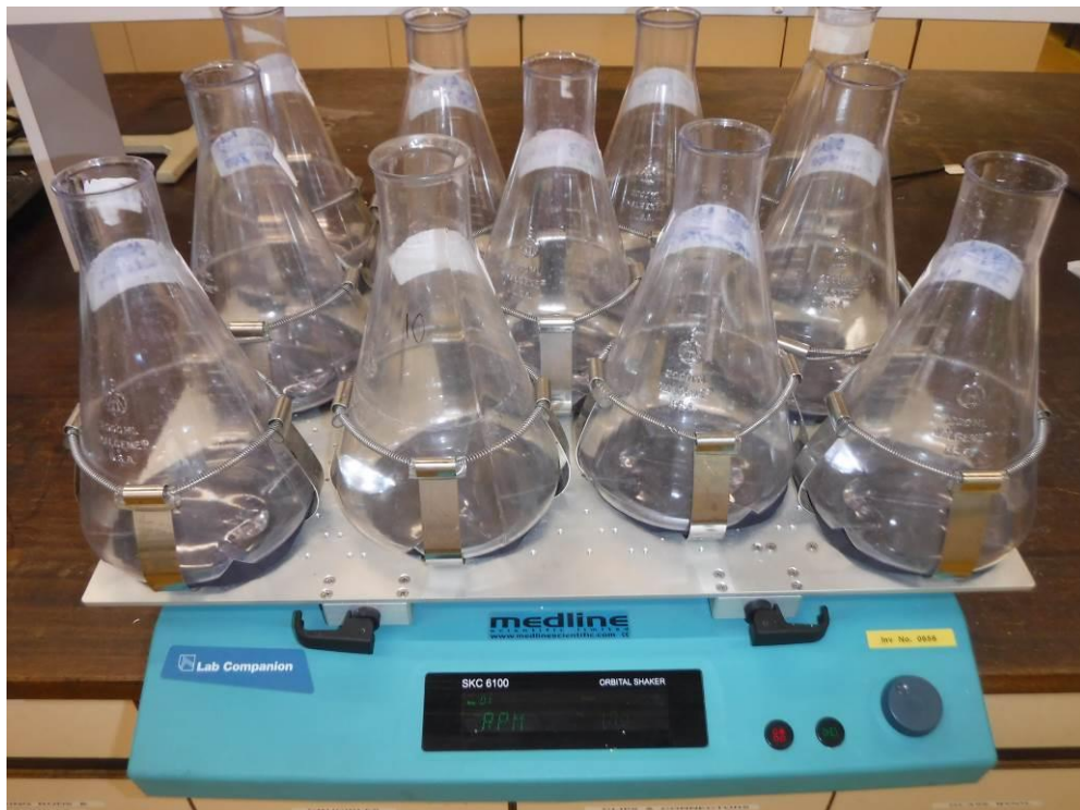
Photograph C 1 Orbital shake table
