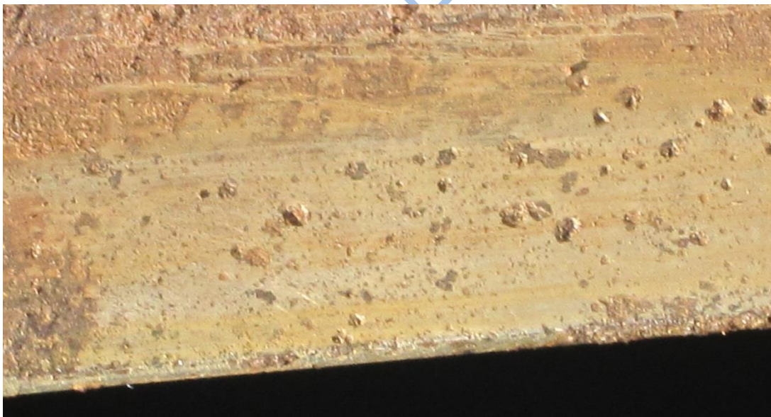
Figure 5-1 Pitting of 304L
