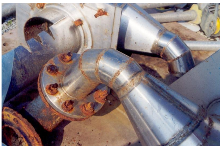
Figure 5-3 Heat tint and galvanic corrosion (© Roger Francis)
