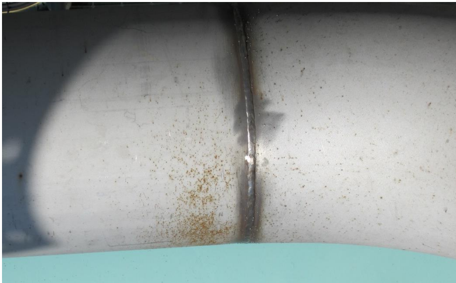
Figure 7-3 Corrosion of weld spatter (© Roger Francis)
