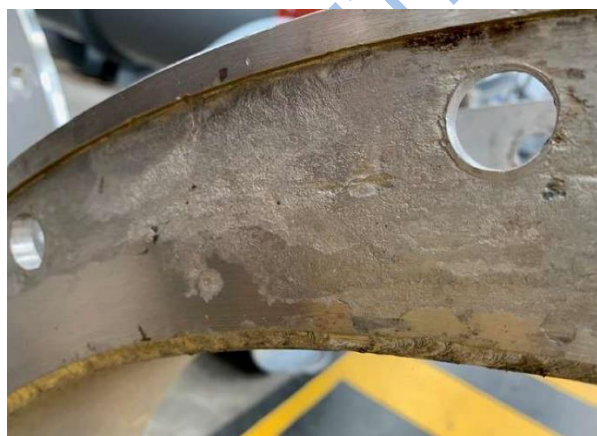
Figure 5-2 Crevice corrosion of 316L (© Roger Francis)
